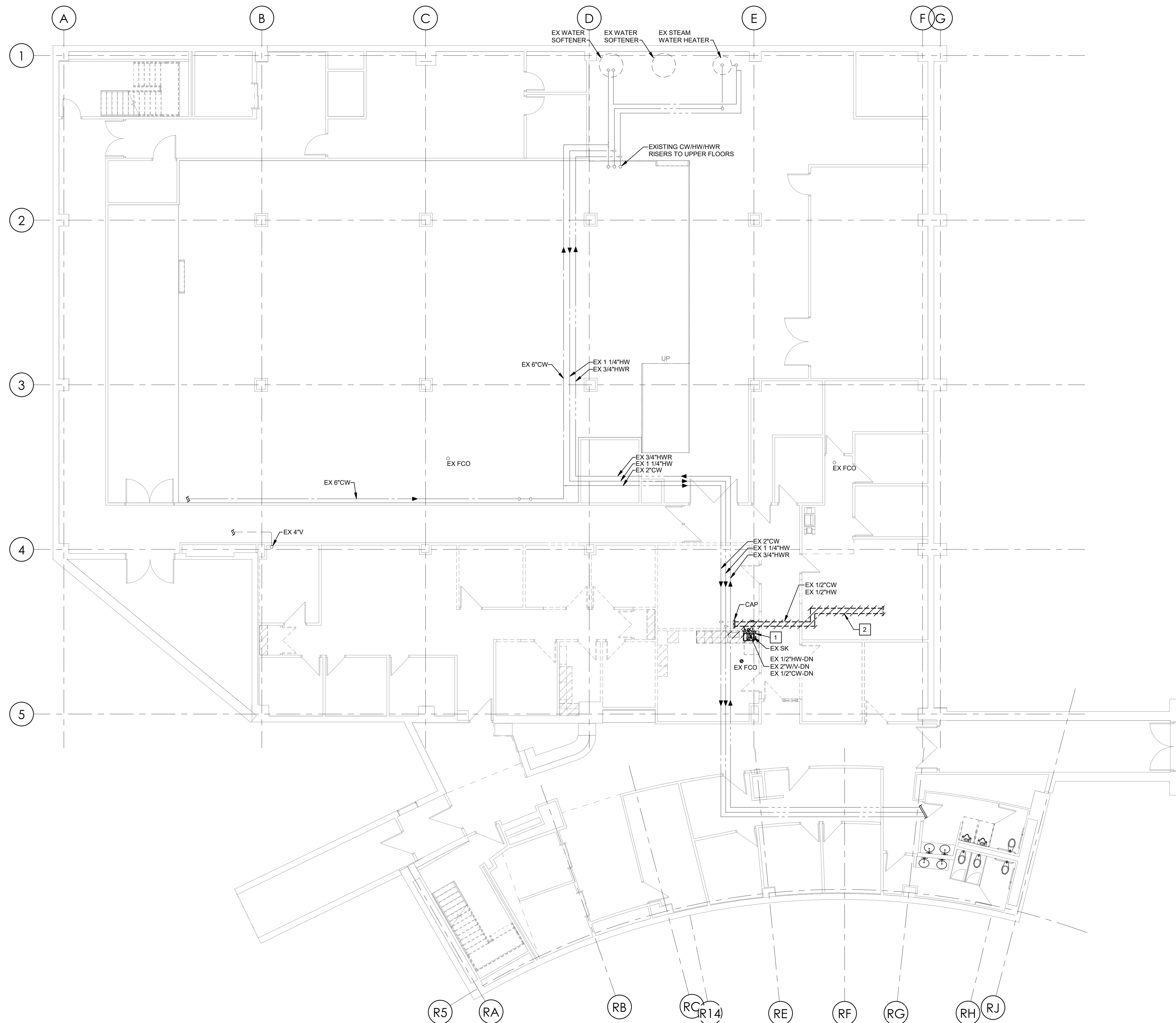
1 PLUMBING - GROUND FLOOR DEMO PLAN 1/8" = 1'-0"
