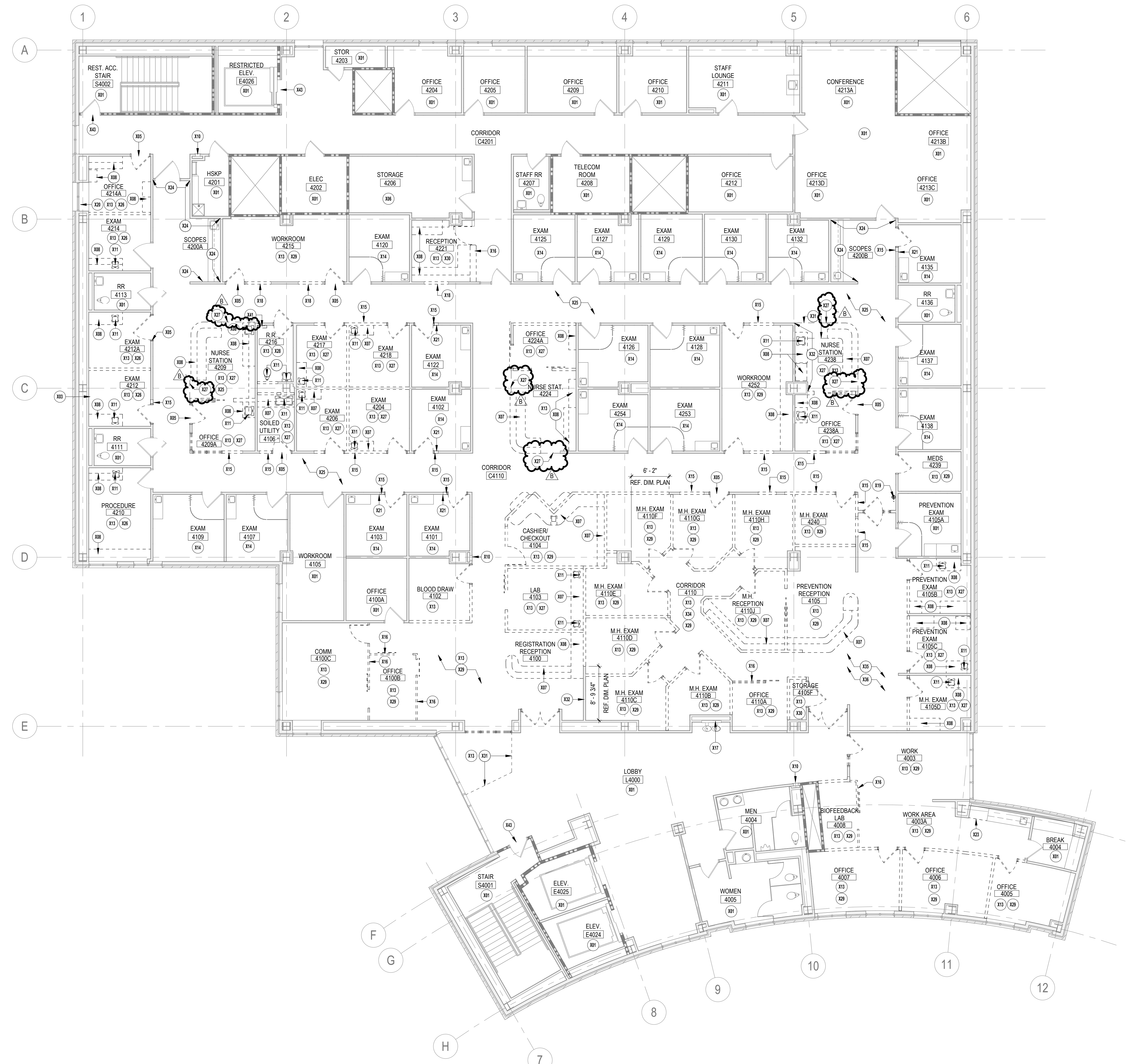
1 FOURTH FLOOR DEMOLITION PLAN 1/8" = 1'-0"
