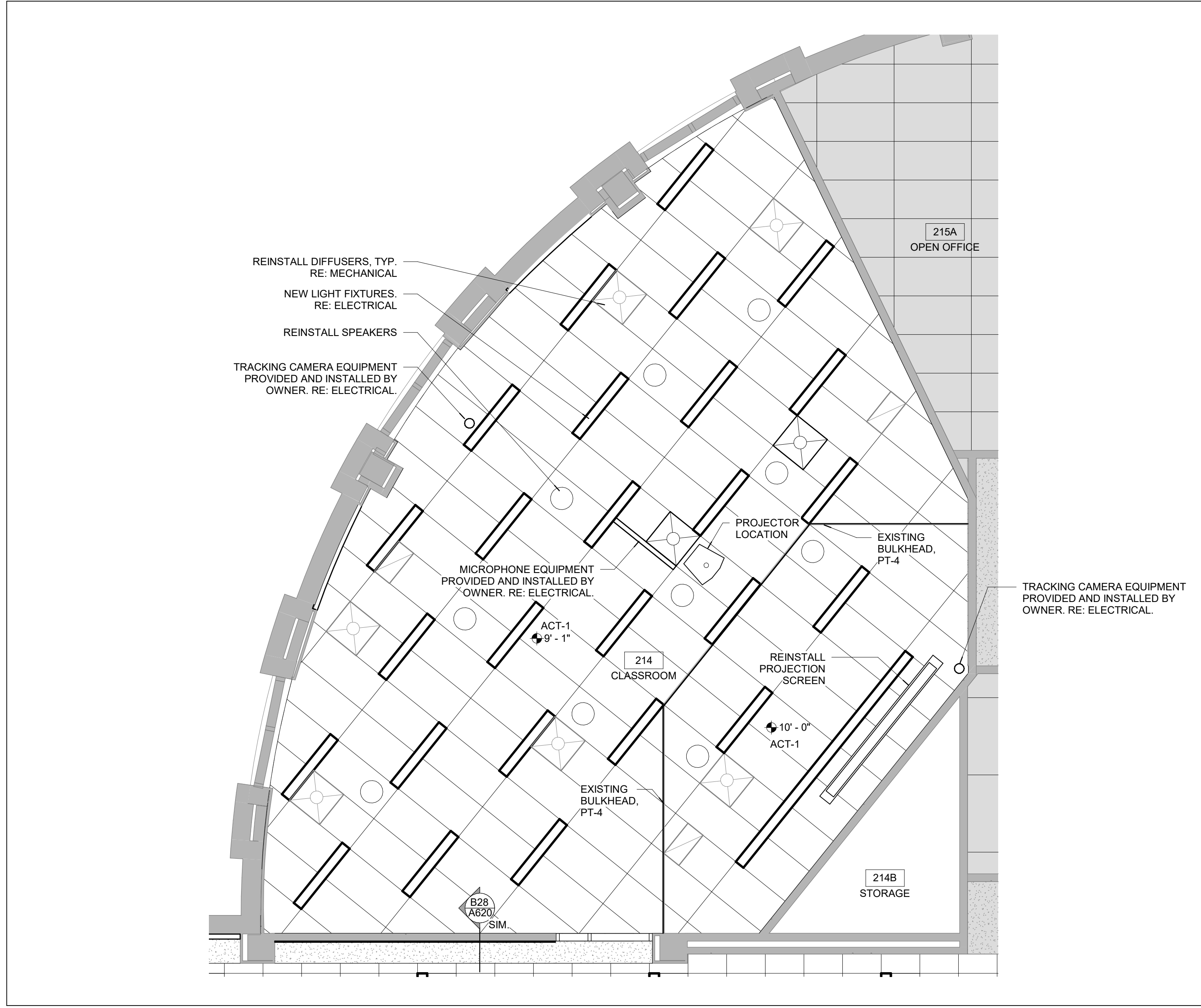
ENLARGED CEILING PLAN - CLASSROOM B21 SCALE: 1/4" = 1'-0"
